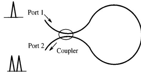
Fig. 1. Simple fiber loop configuration.
