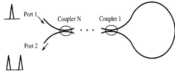
Fig. 4. Multiple cascaded coupler loop configuration.
