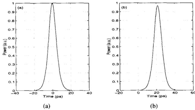
Fig. 3. (a) Input pulse with pulse width = 10 ps, and (b) output pulse after single coupler loop with  $\Delta f = 8$  nm.
