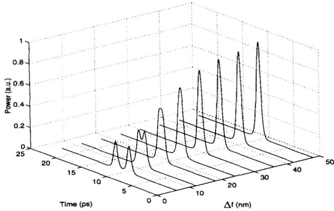
Fig. 2. Output optical pulse with single 3-dB coupler against different  $\Delta f$  with input-pulse width = 1 ps.
