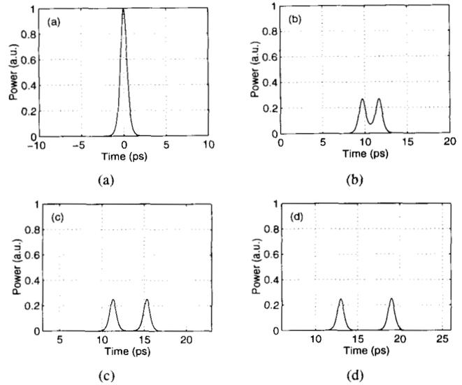
Fig. 5. (a) Input-optical pulse with 1-ps pulse width. Output-optical pulse with (b) single, (c) two, and (d) three cascaded identical 3-dB couplers, each with  $\Delta f = 8$  nm.
