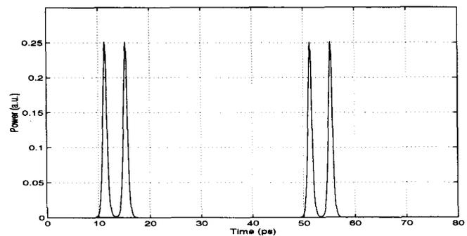
Fig. 6. Multirate optical-clock generation with single 3-dB coupler of  $\Delta f = 8$  nm, input-pulse width = 1 ps and input-repetition rate 250 GHz.
